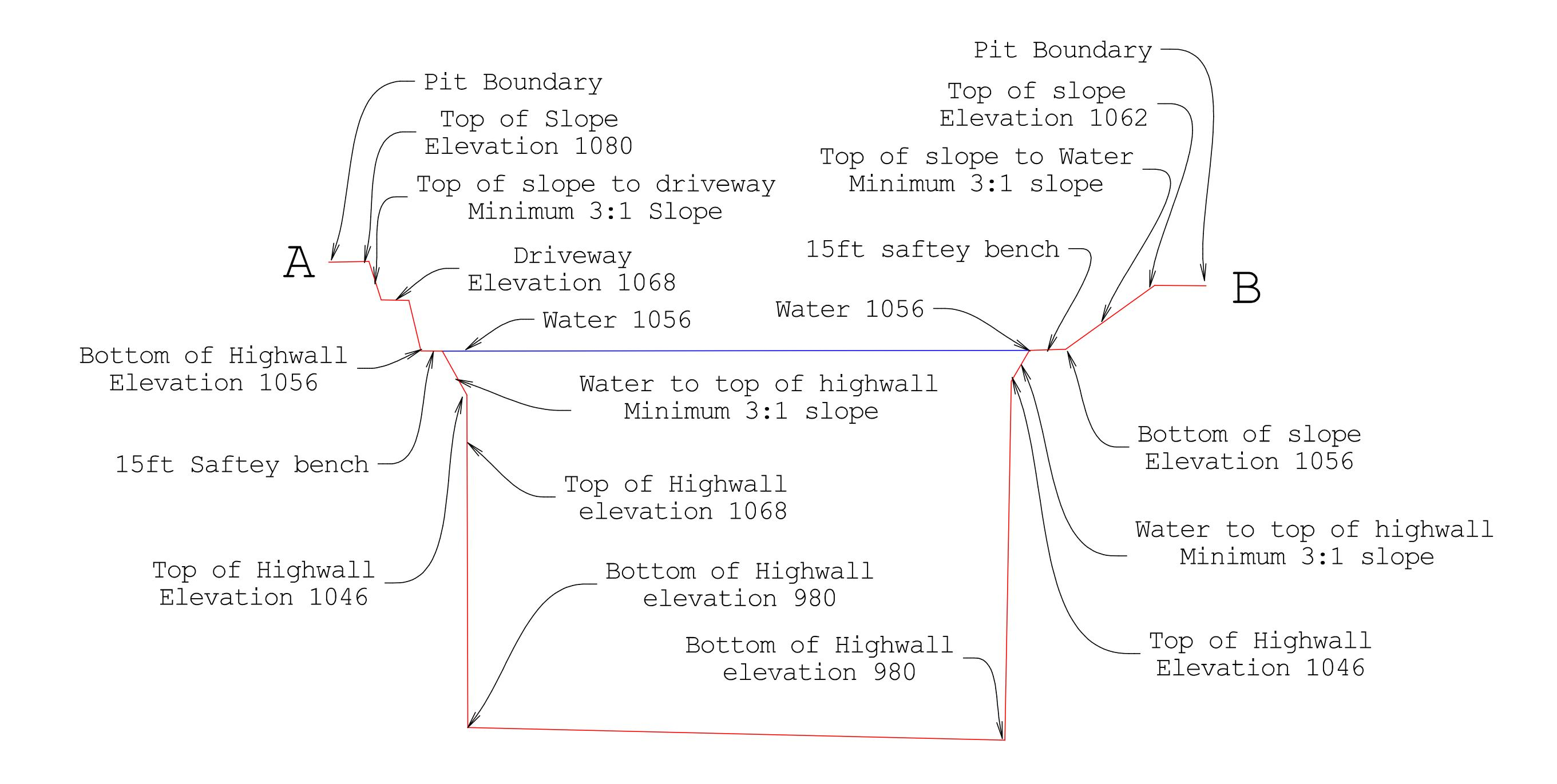
Where vertical walls are proposed to remain below water level, mining operations will not occur in a way that will undercut the vertical wall.
